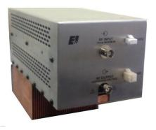
The M-2100-T Amplifier Module is a rugged source of RF power, useful for ultrasonics, laser modulation, RFI/EMI, plasma equipment and general laboratory applications. This module is designed to be integrated in to a system. It requires a DC voltage input and forced air cooling. The M-2100-T represents E&I's commitment to providing RF power amplifiers of the highest quality, durability and ruggedness.
